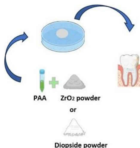
Fig. 1. The schematic illustration of the fabrication method of glass ionomer cement
